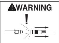
Always disconnect air from nailer/ stapler whenever servicing! During maintenance, a nailer/stapler connected to air may fire accidentally, causing serious personal injury!
